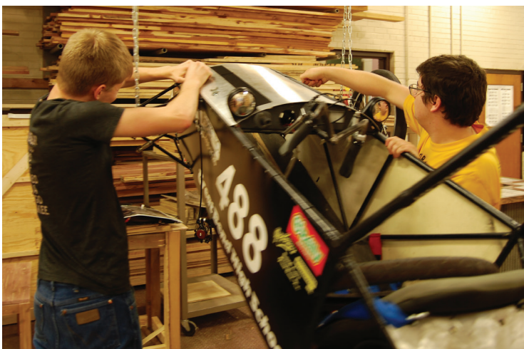
Jace Schwager and Jared Divis take the hood off of the 488 car so they can install the batteries.
